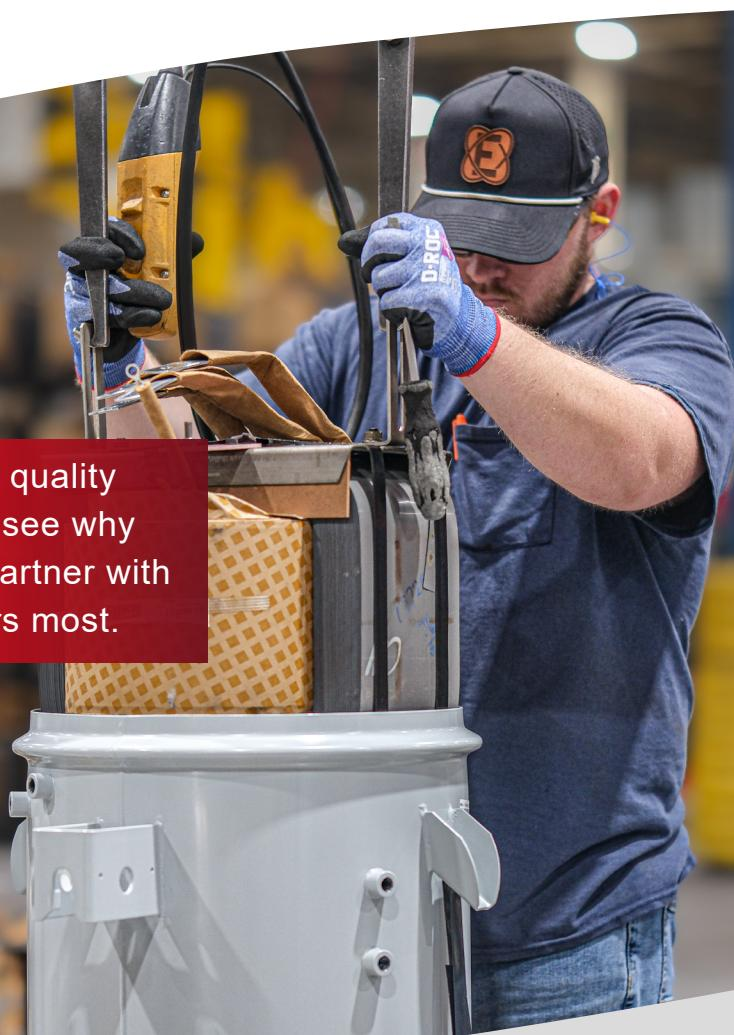
ERMCO's Single Phase Pole Mounted distribution transformers are designed and manufactured in compliance with all applicable IEEE and RUS standards. All transformers are oil-filled, 65°C rise, and designed for usual service conditions per IEEE C57.12.20.
