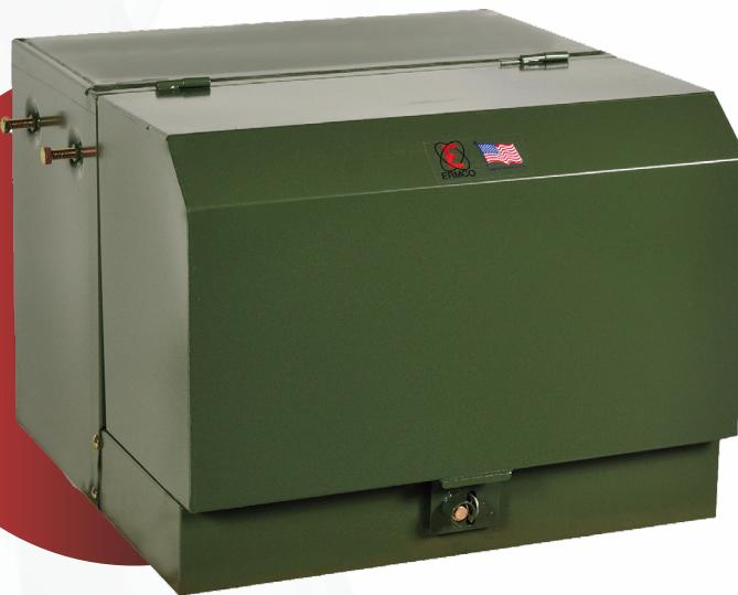
ERMCO single phase pad mounted distribution transformers are designed and manufactured in compliance with all applicable IEEE and RUS standards. All transformers are oil filled, 65°C rise, and designed for usual service conditions per IEEE C57.12.00.
